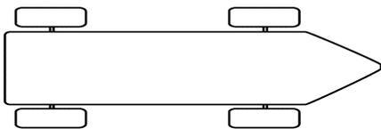
If the front of your car is shaped to a pointed, it will not rest against the starting pin and it may not trip the timing sensor immediately at the finish line.
